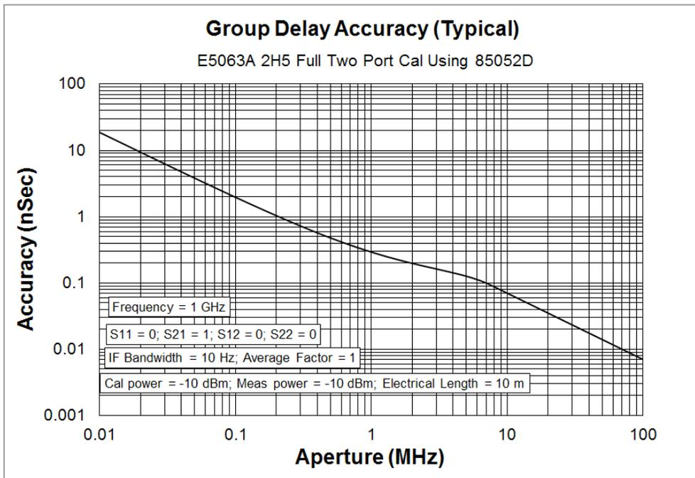
In general, the following formula can be used to determine the accuracy, in seconds, of a specific group delay measurement:
